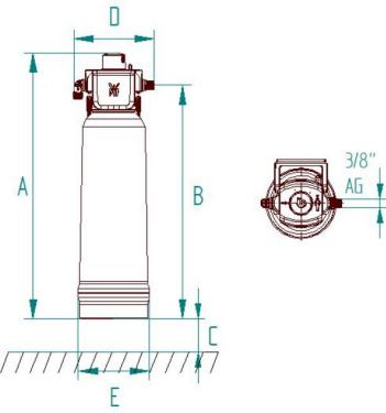
It is recommended to plan with the dimensions of a 2 XL filter cartridge as the water quality varies from location to location
